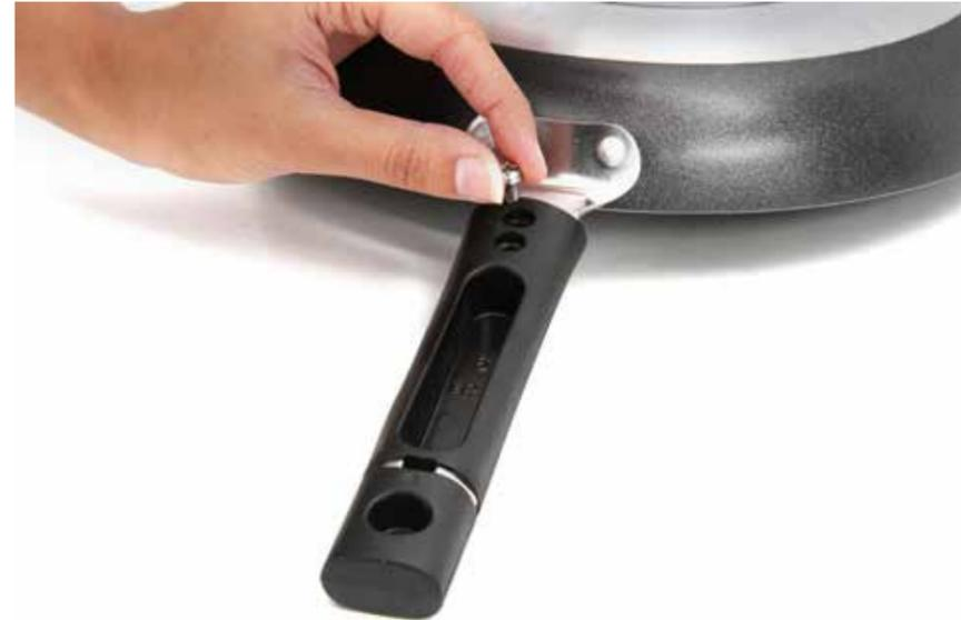
Turn the tawa or pan upside down and hold the handle to the already riveted handle spur such that the screw holes on both are aligned. Place one screw each in the two holes.
